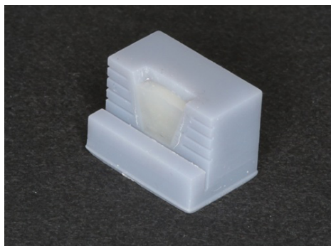
Fig. 4. Plastic mold with a trapezoidal slot filled with the bottom horizontal layer ~ 4 mm.
