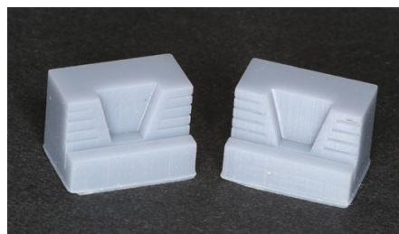
Fig.1. Plastic molds with trapezoidal slots for a composite material.
