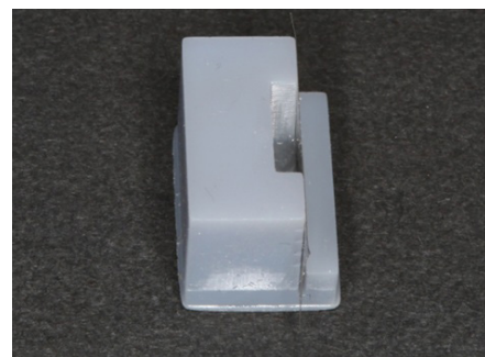
Fig.2. Plastic mold with a trapezoidal slot covered with a metal strip.
