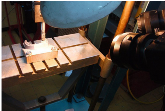
Fig. 2A. The control cast under the load in a dynamometer.
