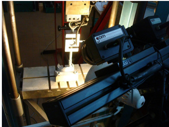
Fig. 2B. Measurement of the force applied to the coping model.
